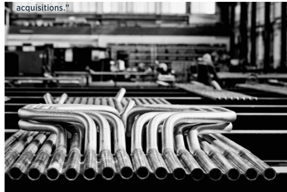
Pipe bends as part of a replacement of boiler pressure parts
