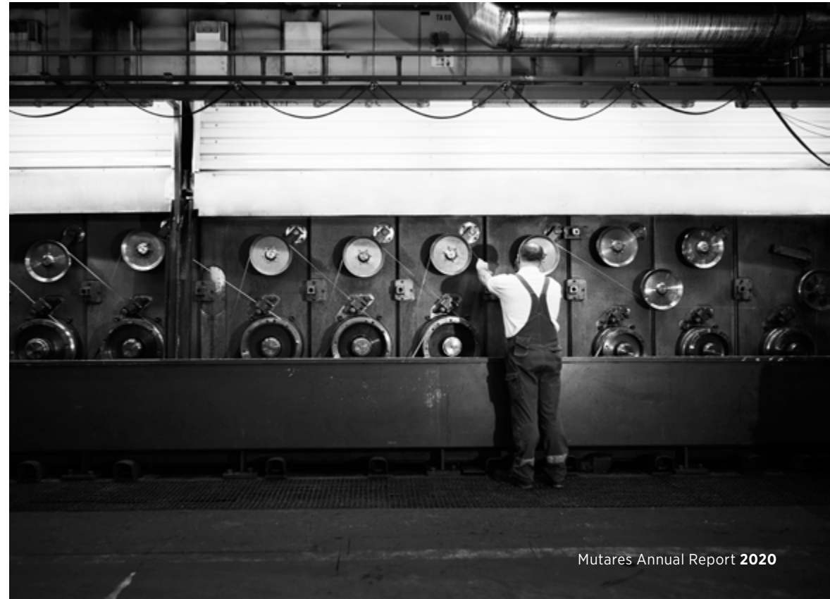
Employee checking machine, which is making copper wire thinner by extending it
